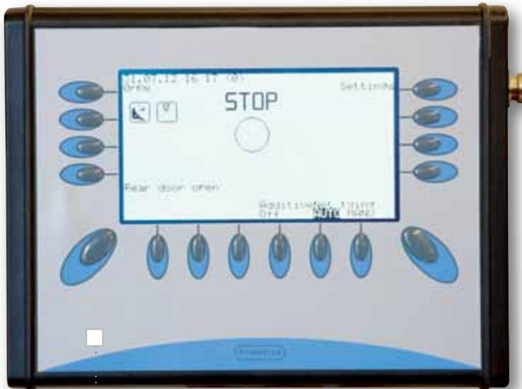
..... The screen of the control display contains an info and a setting section, and big letters make it easy to read the information provided in both sections during day and night operation.
