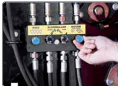
All hydraulic functions are grouped on the left-hand side of the baler, so checking and adjusting can easily be performed by a single person.
