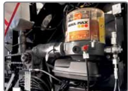
Hydraulic oiling and central greasing canisters are placed at eye level for easy checking in an uncluttered area for easy refilling, without spillage.
