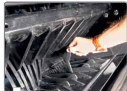
The knives are checked and replaced without any tools – quick and easy.
