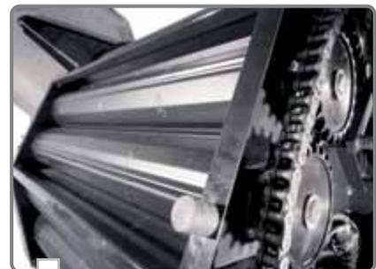
The support bushes for the compression rollers are fixed with two bolts. In case of a replacement, this can be done without removing the roller.
