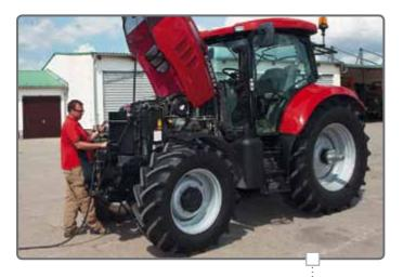
Easy daily checks and cleaning: with new ....... swing out coolers. Similarly the air filter is conveniently situated for quick inspection. Should you only be checking the oil level, this can be done with the hood closed.
